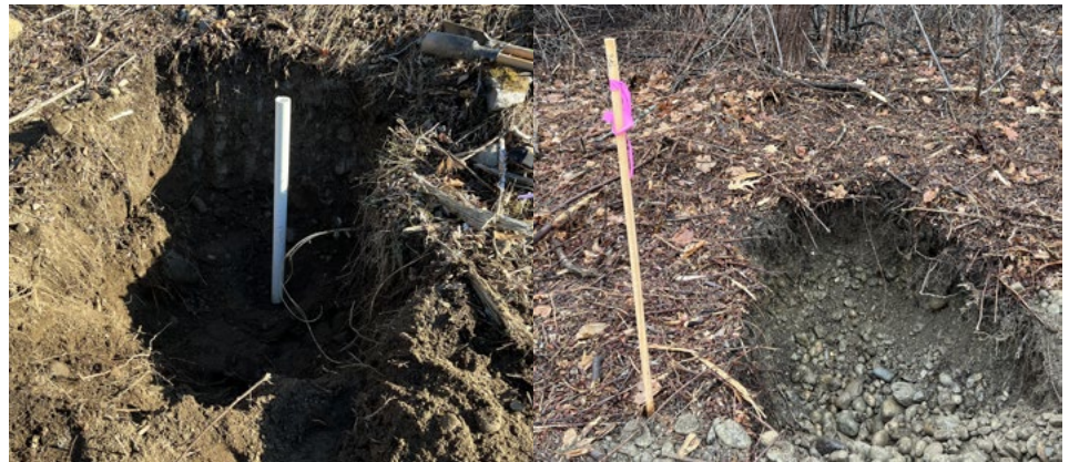
Photo Caption: Test pits and monitoring well to test percolation rates for onsite manganese residuals management.
